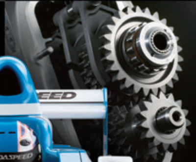
Hewland FTR 6-speed sequential gearbox with no-lift shift
